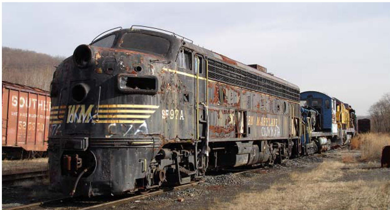
Near the yard's entrance rests one of the quintessential freight and passenger locomotives, the F-7. Time has been quite unkind to this locomotive; in numerous places the body has rusted straight through. Spray-painted on the nose is CNVX no. 97A.
