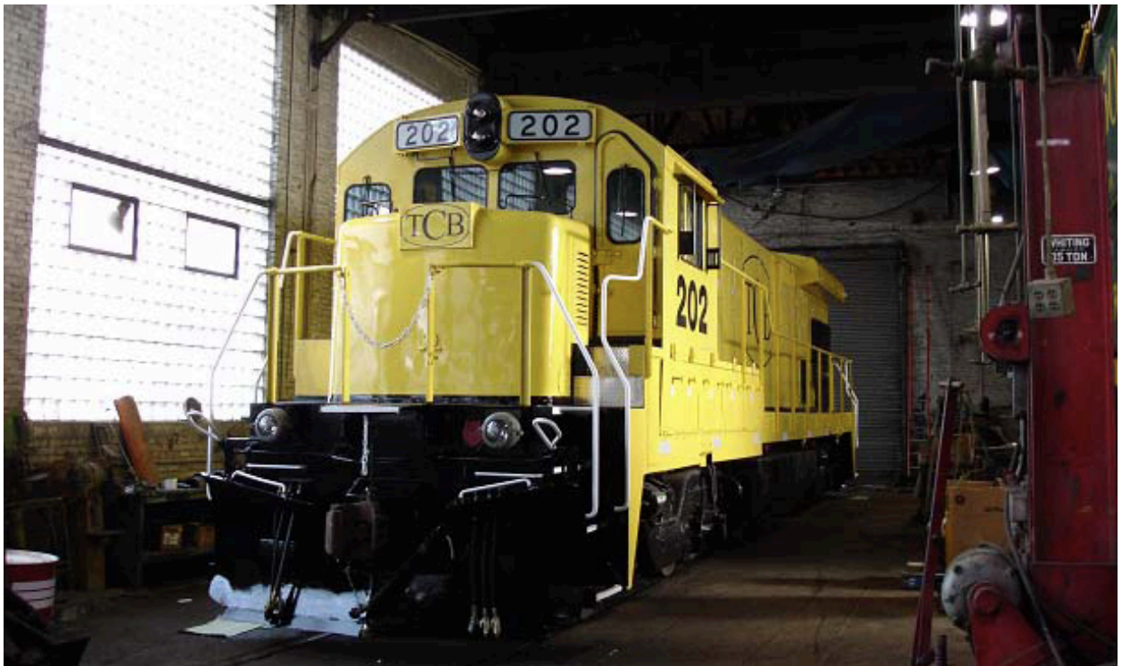
Inside the diesel shop (and Ronald M. Delevan, Inc.'s headquarters), a Texas Central Business Lines 4-axle GE nears completion. Note the diamond-plate steps to the cab door.
