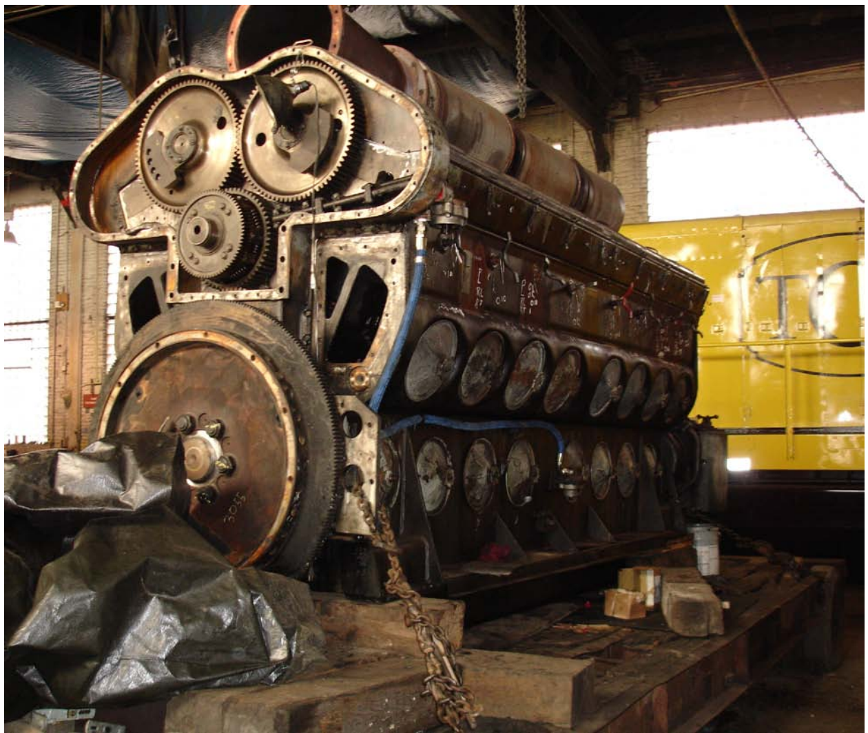
Also to the right of the Texas Central Business Lines GE is a prime mover. As indicative of its size, note that it rests on a semi trailer.
